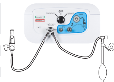
Fig 2. Bagging System connections
